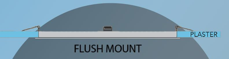
Our most popular style of illume is the "FLUSH" mount option, as it is the same thickness as your plaster. Making it easier to install any where! The illume is even IC-4 rated, which means you can cover your illume with insulation bats!
