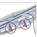
Use 2x coach screws to secure bracket panel in place. (Do not use screws as a clamp)
