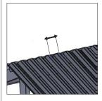
Measure roof corrugations before attaching brackets to the solar collector. Brackets should be attached to the top part of roof corrugation, not in the valley.
