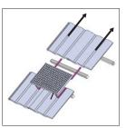
Slide roof tiles up (Remove if necessary) to install panel. Place panel in position.
