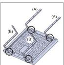
Align brackets to unit with roof pitch and use (6mm) Nuts and Bolts with 4x washers to secure (A) & (B) Brackets in position as per the diagram.
