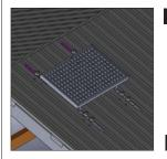
5 Fix solar panel to top of roof, with cable fitted underneath ridge cap. This eliminates the need to drill a clearance
