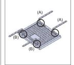
Align brackets to unit with roof pitch and use (6mm) Nuts and Bolts with 4x washers to secure (A) & (B) Brackets in position as per the diagram
